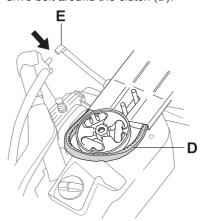
Pull off the cutting arm by pulling it straight forwards, as illustrated.
